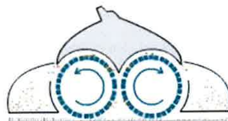
Twin Cylindrical Counter rotating brush machine cross section
