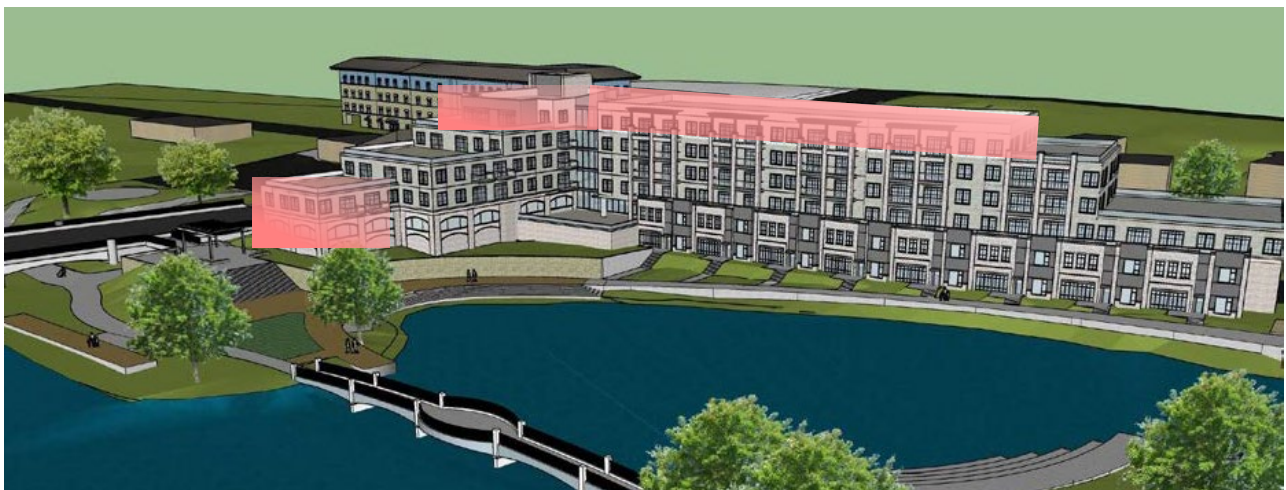
Figure 1: 4-Story Modification of Charrette Final Recommendation: Fifth floor apartments and 2-story wing (shown in pink) were removed for this analysis
